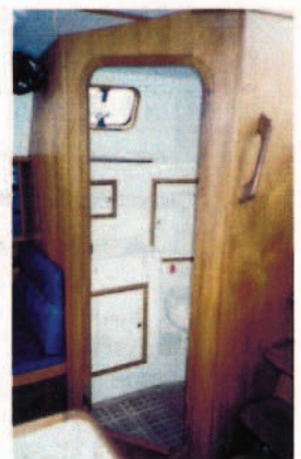
Aft head has large wet locker
