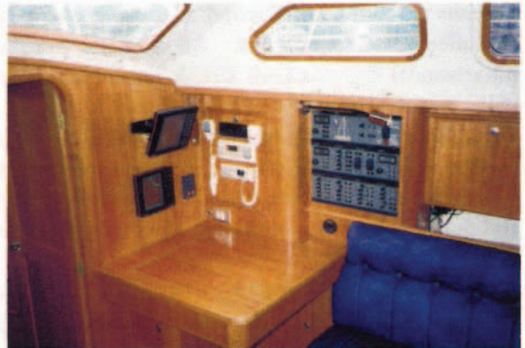
Half size chart table accommodates full electronic instrumentation
