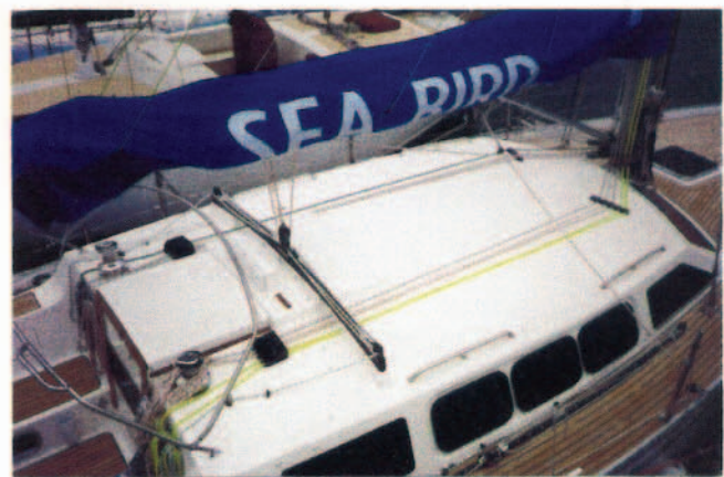
Control lines lead aft to cockpit through rope jammers
