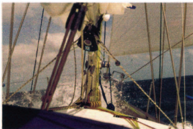
Boom brake acts as a preventer and friction brake
