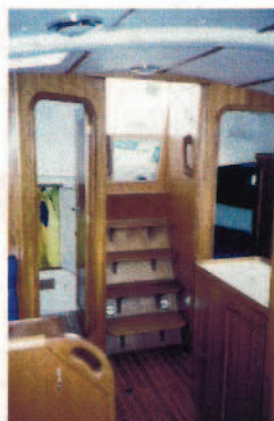
Companionway steps lift up to access engine
