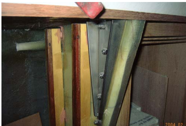
Solid glass chainplate knee detail.
