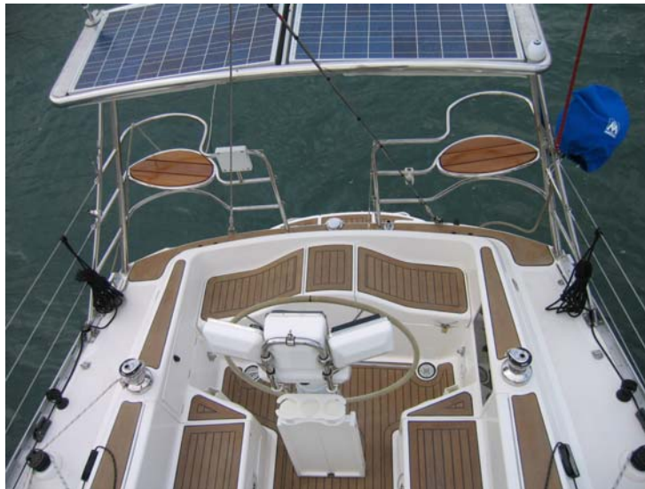
Pushpit arch incorporates transom seats, bimini solar panels, davits, outboard mount, and bbq.
