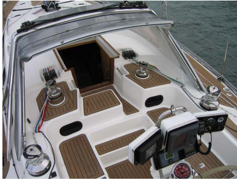
Mast controls lead to cockpit halyard winches.
