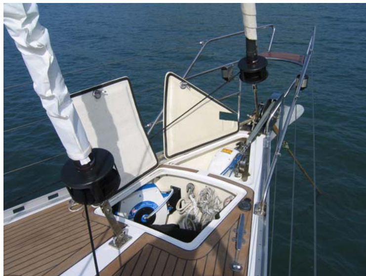
Windlass is mounted below deck. Extra foredeck storage locker houses fresh / saltwater deckwash hose reel.
