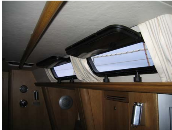
Opening ports in main cabin for crossflow ventilation.
