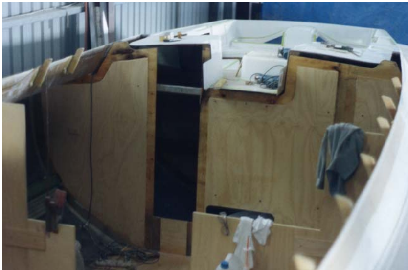
Structural plywood bulkheads being fitted.
