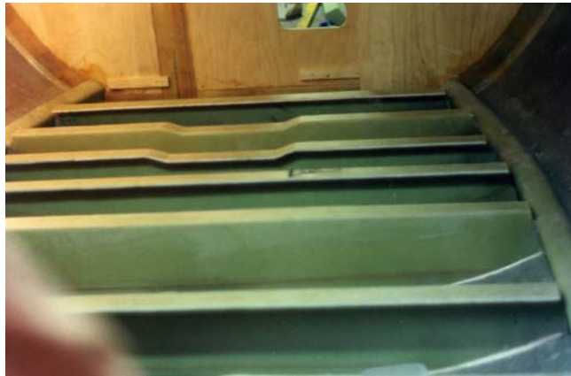
Solid glass structural floor members.
