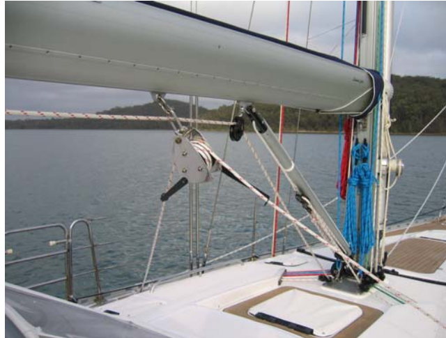
Boom brake arrangement.
