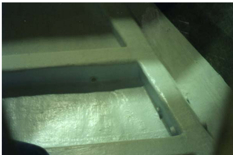
Forward cabin under floor hull stiffening.
