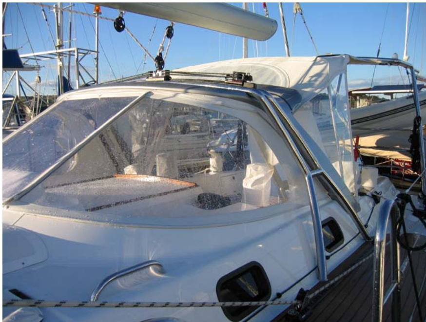
Standard dodger incorporates mainsheet arch.
