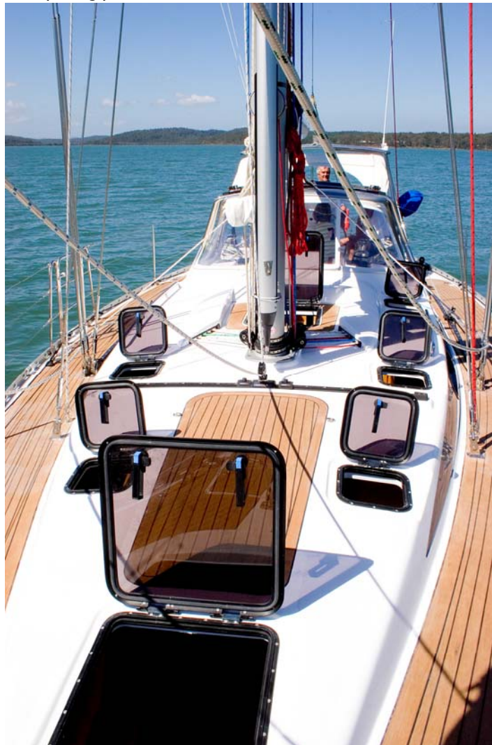
7 deck hatches for flow through ventilation.
