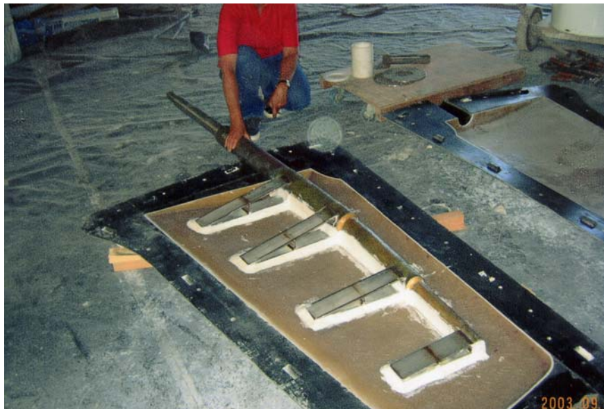
Rudder shaft is wrapped in GRP then bogged into position.
