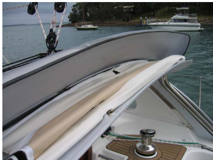
Pushpit arch incorporates transom seats, bimini solar panels, davits, outboard mount, and bbq.
