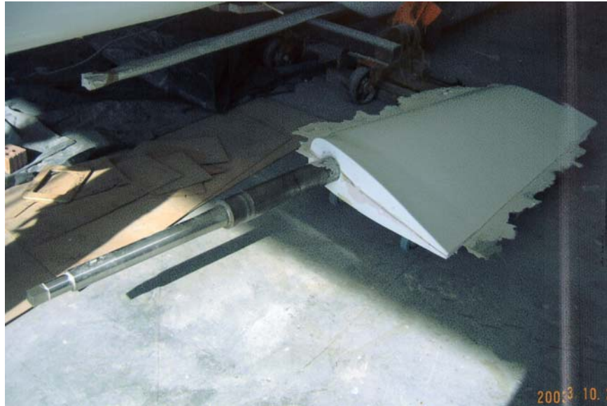
Joined rudder. Note excess filler has squeezed out ensuring no voids are left.
