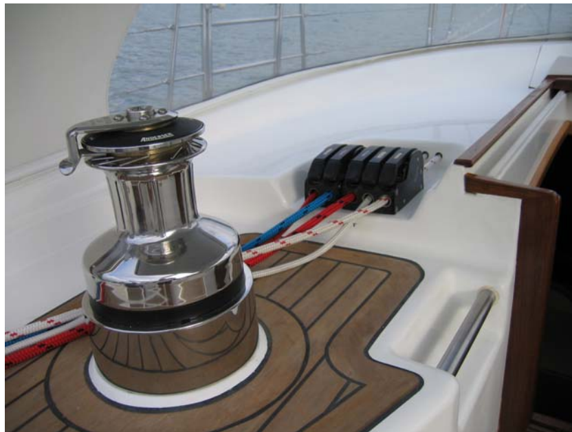
Cockpit controls leading back to Andersen 46 ST electric winch.
