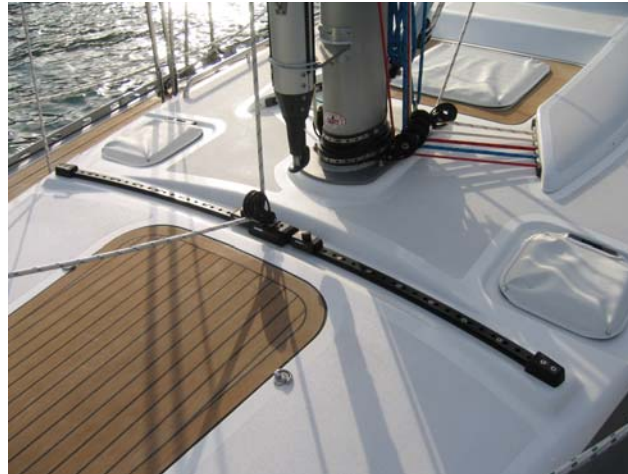
Self tacking arrangement.
