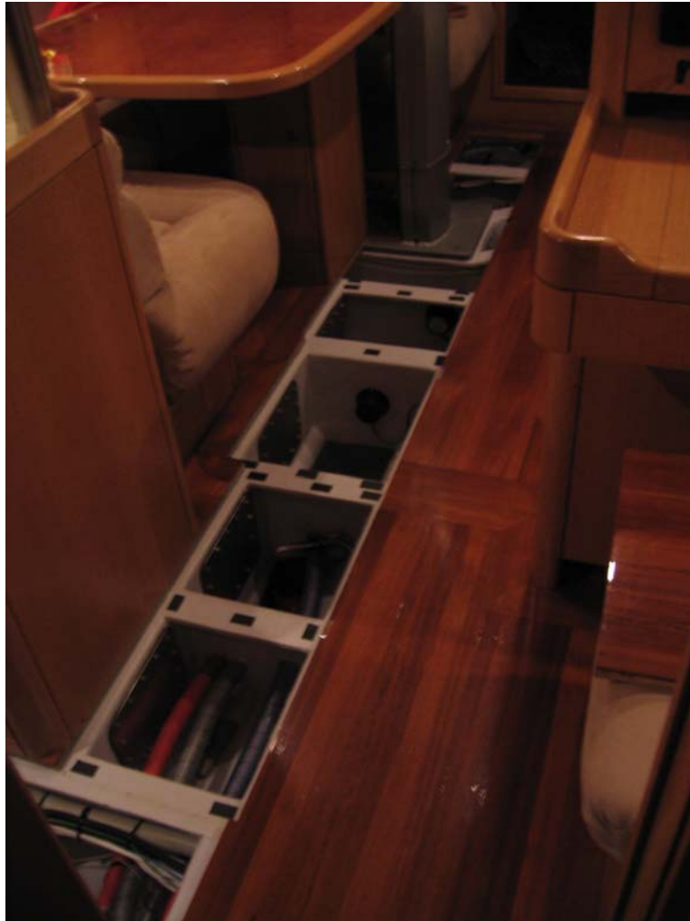
Access to keel bolts / main bilge.
