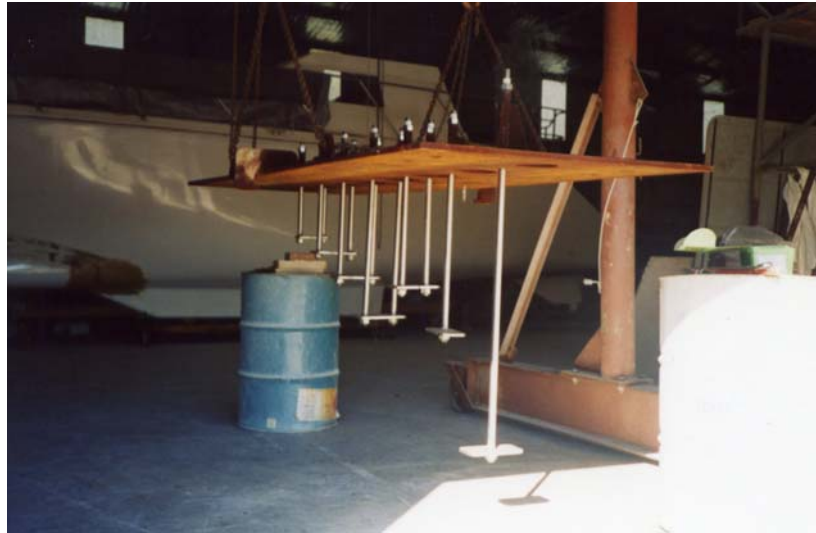
Keel bolts set at varying depths.
